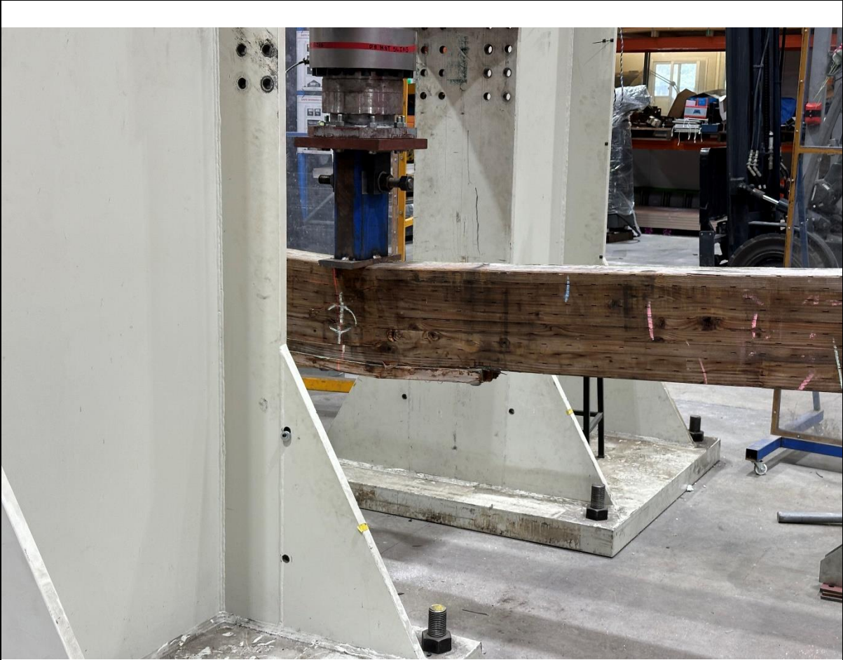
Testing the capacity of a repaired beam
