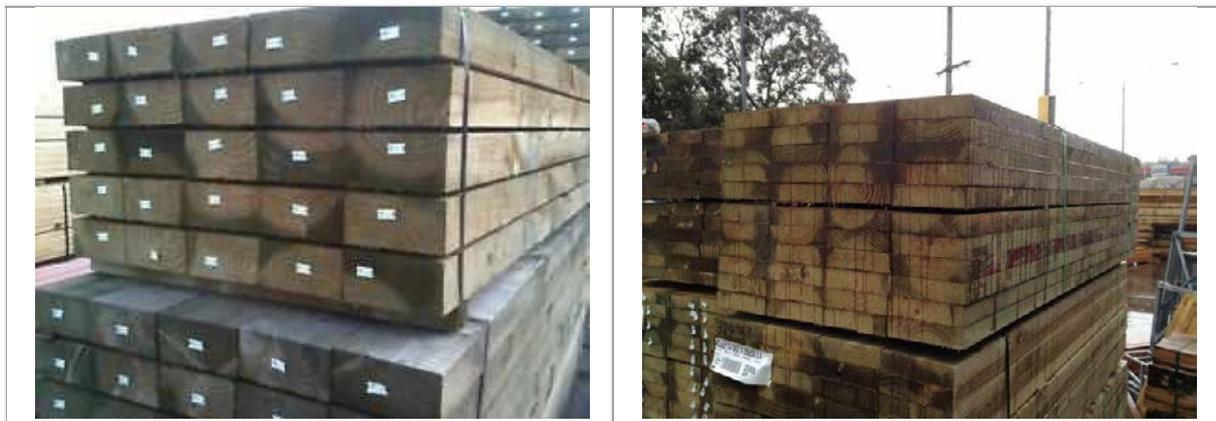
*Images of badly treated sleepers taken from resellers websites, they think they are good **Just a tip, the dark bits are the areas that are treated, should be 80% of the cross section.***
