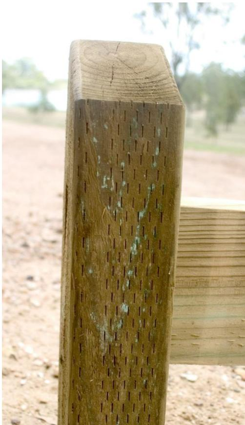
If I was purchasing significant amounts of pine I would require the timber to be preconditioned, incised to a depth of 10 mm and treated preferably to H4. The incising process allows the chemicals to penetrate the heartwood and the extra chemical cost for H4 is not significant when weighed against the cost of failure. Many Australian purchasers do not know what incising is and the image on the left shows what incised timber.
