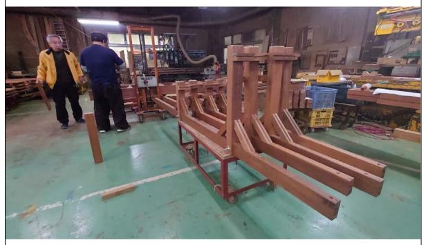
The deck was precut and partially assembled in the factory under a controlled environment and the scrutiny of the Kuratas. They were previously furniture manufacturers and everything is done with that level of precision and quality. the timber quality is similar to that in the first article. Kurata Co order well and their miller knows their expectation.
