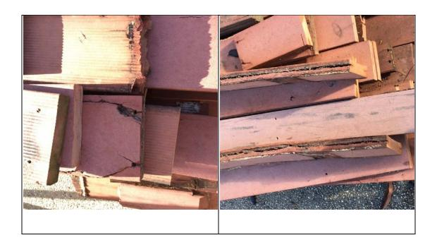
One of my readers sent me these images of a well known brand of plastic timber composite decking. The deck had failed for the second time and was being replaced with timber. Most of us would not go back for a second helping. The builder noted when the decking split it swelled and locked in water which eventually attracted termites, note on the photos the splits in the sides of the decks which are cupped, split etc.
