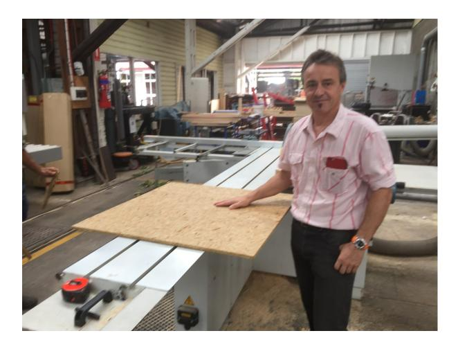
This sheet is an original attempt to produce a prototype building panel manufactured from agri-fibre, in this case sorghum stalks. Similar experiments with sugarcane bagasse performed by FPI crew showed boards could be produced with better properties than standard particleboard. Utilisation of these by-product fibres could become very important in the future.
