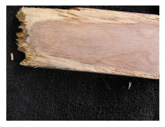
Not all sapwood is lyctus susceptible and doesn't get turned to powder from the larvae but that does not change the fact that it is not durable if used externally. The image above shows decay in blackbutt sapwood. When the piece was freshly cut the sapwood is clearly visible
